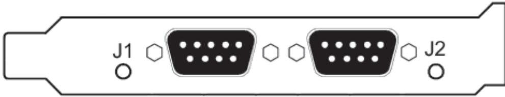
The connection of the networks is made by means of an RS-485 serial cable, directly to connectors “J1” and “J2”.
