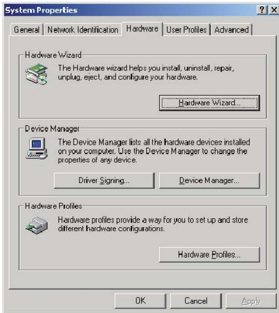
When you click on the “*Device manager*” (or “*System*”) key, the window shown below appears. Expanding the “*Ports (COM & LPT)*” item, the new COM port installed with the isa card is included: Windows calls it “*Communications Port*”.
