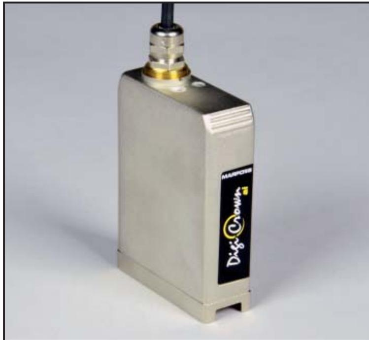
The *DigiCrown ai* module has been developed for managing analog inputs (tension or current) to the DigiCrown system. Through this module it is possible to integrate in the network third-party sensors such as load cells, torque sensors, flow-meters, pressure and humidity sensors.
