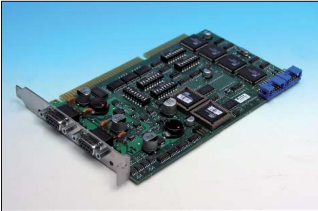
The *DigiCrown isa* unit achieves the RS485 Half Duplex serial communication with the rest of the network. Each card is equipped with two serial ports, for the overall management of 31 + 31 sensors or I/O modules.
