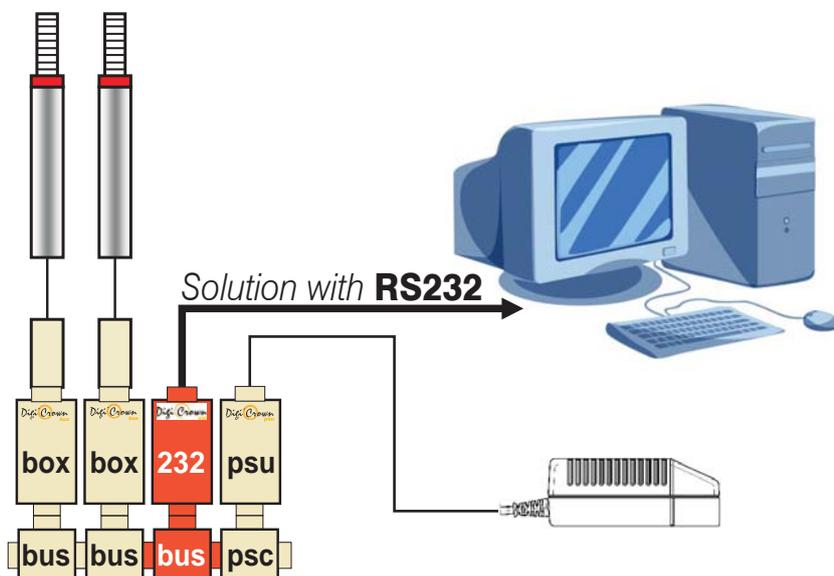
The **232** module is fitted on the *DigiCrown bus* unit, by means of which the communication with the data acquisition system takes place. The **232** module supplies to the *bus* connector a square wave with a 75 KHz frequency, for the generation of the sine wave that synchronizes the transducers. The connection to the *bus* module is made via a 9-way sub D-type connector, which also supplies power to the **232** module.
