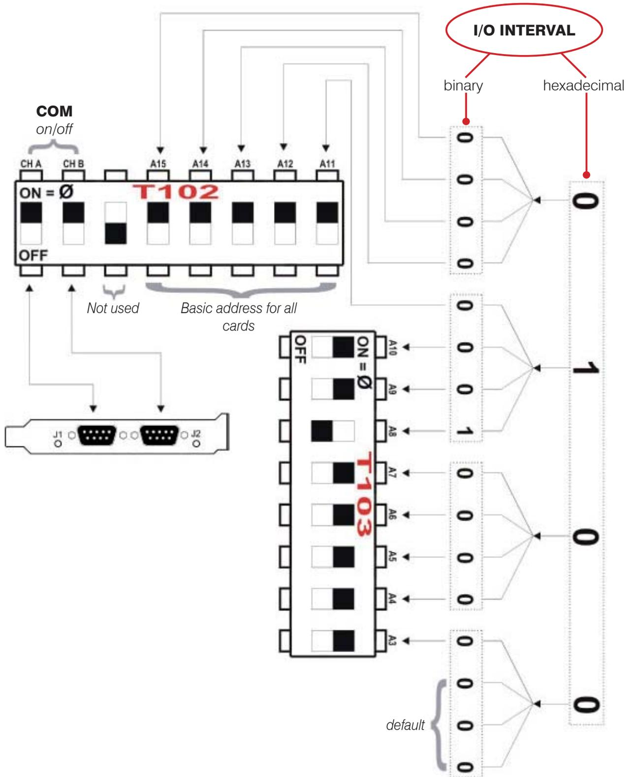
In order to simplify this operation, and reduce the risk of errors to a minimum, a “CONFIGURATOR” is provided in Excel format that allows the user to define the position of the dip-switches graphically, based on the hexadecimal values defined using the Windows installation procedure.
