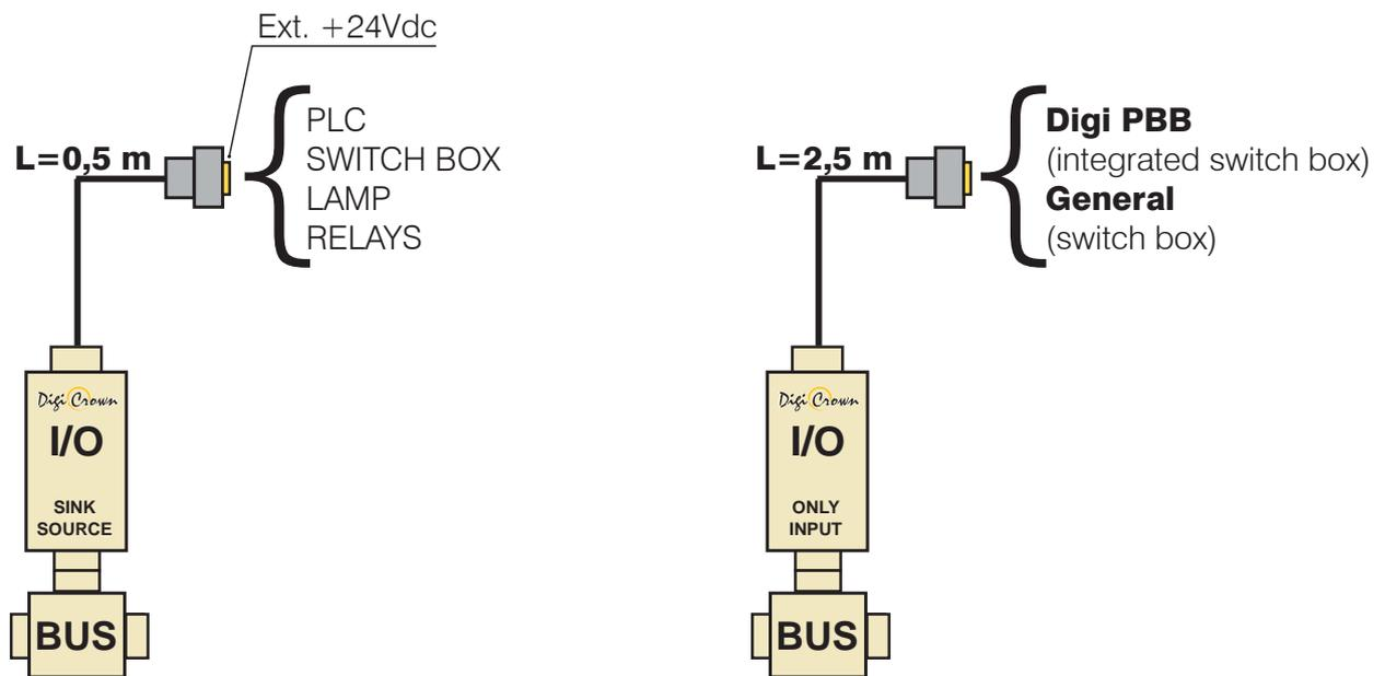
The **I/O** module is mounted on the *DigiCrown* **bus** unit, which is used for communication with the data acquisition system with a standard RS-485 serial connection.
