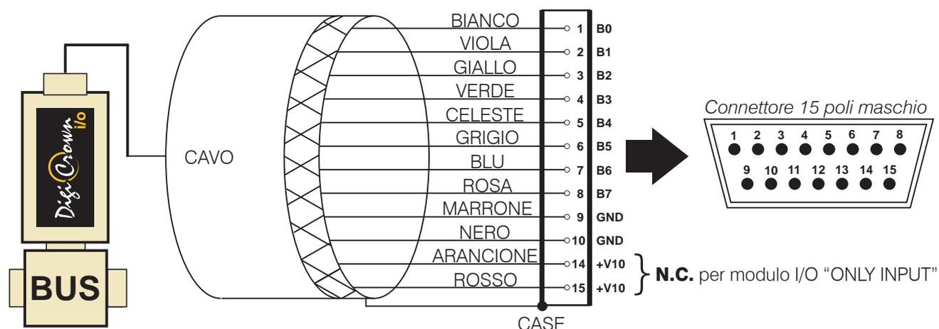
Pins 1 - 8 of the 15-pin male D-sub connector are used to connect the **I/O** module to external signals.
