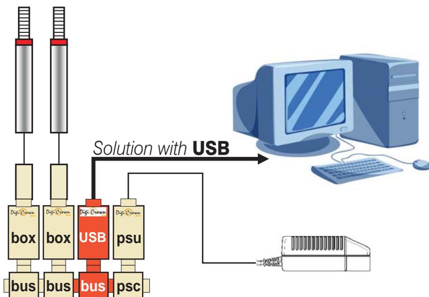
Installing *QSPC*, *Easy Acquisition* or the *Marposs Driver Library*, will allow the automatic detection of the **USB** unit as soon as it's plugged to the host PC. As soon as Windows finds the new hardware connected, select the option "Install the software automatically" and click on "Next" (fig. 3). The driver for the **USB** unit will then be installed.
