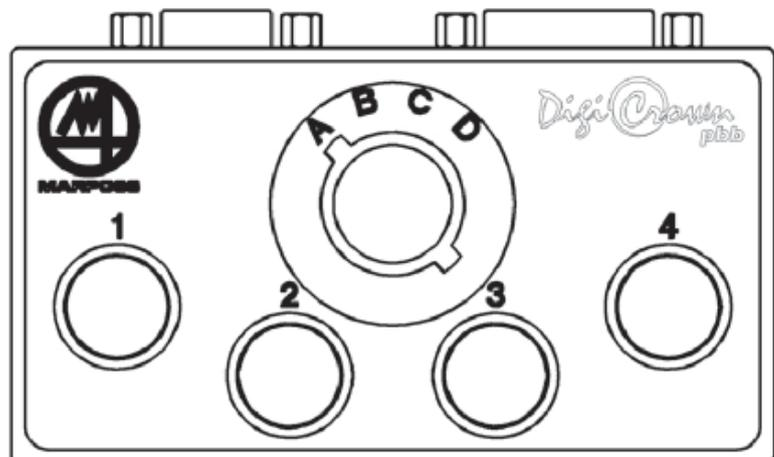
(\*) The bit 4 reserved to the “D” position of the selector, it’s automatically assigned to the footswitch by unscrewing the 9-pin male connector.
