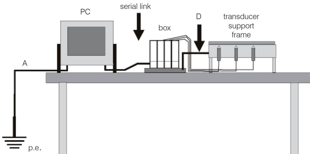
The “D” equipotential connection between the box modules and the transducers support frame, can be done whether a metallic conductive frame is used. In the glass gauging applications the transducers support frame is usually not a conductive material and the transducers are typically insulated, in this case no ground connection is required.
