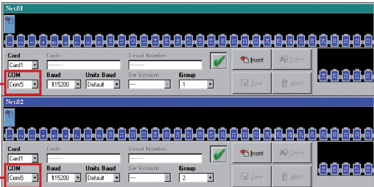
The number of COMs assigned by the PC in the “*Device Manager*” window (COM5, COM6, etc.) is the same that must be entered in the “*MDHQSPC*” configuration software.
