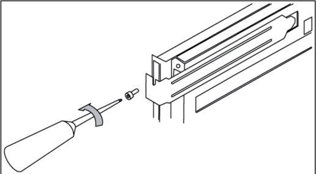
Insert the card in a free PCI slot.
