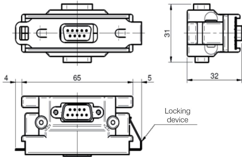
Hooking of box module to bus connector.
